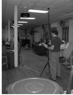
Fig. 10. Measuring UVGI fixture output to ensure effective level of UVGI using a radiometer fitted with a 254 nm sensor. Source: TUSS Saint Vincent's Hospital, Manhattan, NY. Used with permission.
