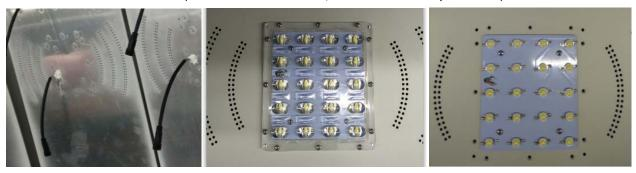
5. Fix the new LED module to the aluminum board, fix the lens (there is a hole on the aluminum board for the module cable to go through )..
