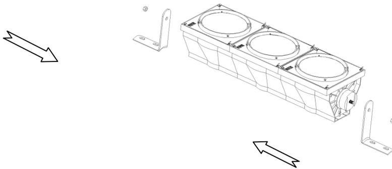
1. Connect the L-shape brackets to the PC modules.
