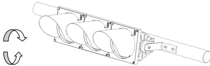
Connect the complete set to the lamp pole via mounting bracket and adjust the angle by the PC modules.
