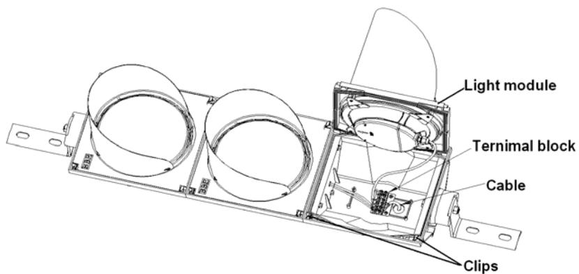
Apply the rubber wire (spec:  $2 \times 1.0 \text{ mm}^2$  VDE 60245IEC57) for out wiring via the hole beside the connection terminal.
