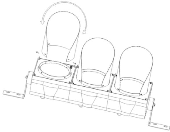
1. Curve the sun visor and insert it in the slot.
